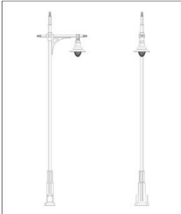
Figure 2.3.3 “Triborough Bridge and Tunnel Authority” lamppost with “Knickerbocker” luminaire.
